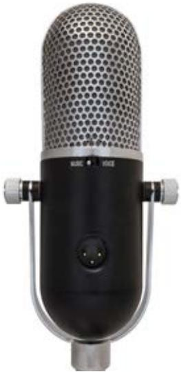
The Heil PR 77 D features a two-position switch allowing the selection of the best characteristics for voice or music. The voice position rolls the audio off at 120 Hz at -6 dB per octave while the music selection removes the filter and the entire audio spectrum of 60 Hz to 16 kHz is present.
