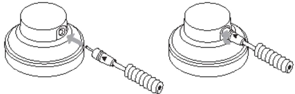
In order to lock your selected cable into the Pro Set 3 you simply insert and twist to lock.
